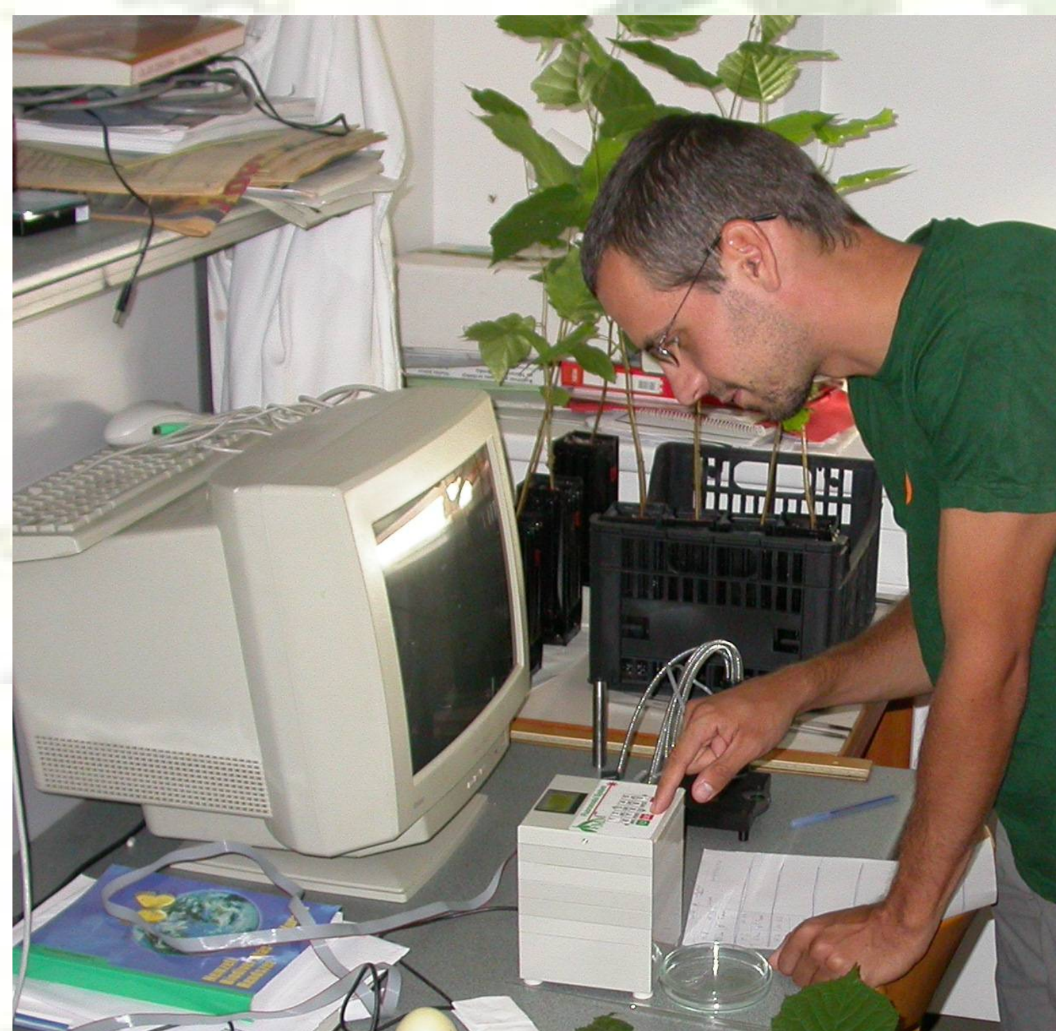
Figure 1. Measurement with FMM fluorometer
